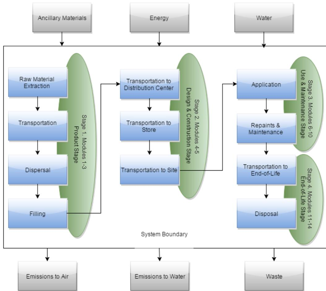
**Figure 1. Diagram of System Boundary for the EPD.**
