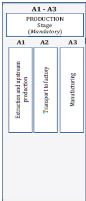
Figure 1. Diagram of System Boundary Covered by LCA Models and Report. Modified from ISO 21930:2017. All other modules were omitted from this study.
