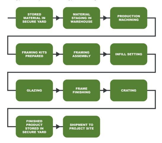
Materials are received into the production site in Lakeshore, Canada where they are stored prior to going to the production floor where the aluminum is cut, fabricated and assembled into frame units. Glazing is then added. Once the frames are finished, the wall systems are packaged and then stored in the yard prior to shipment.
