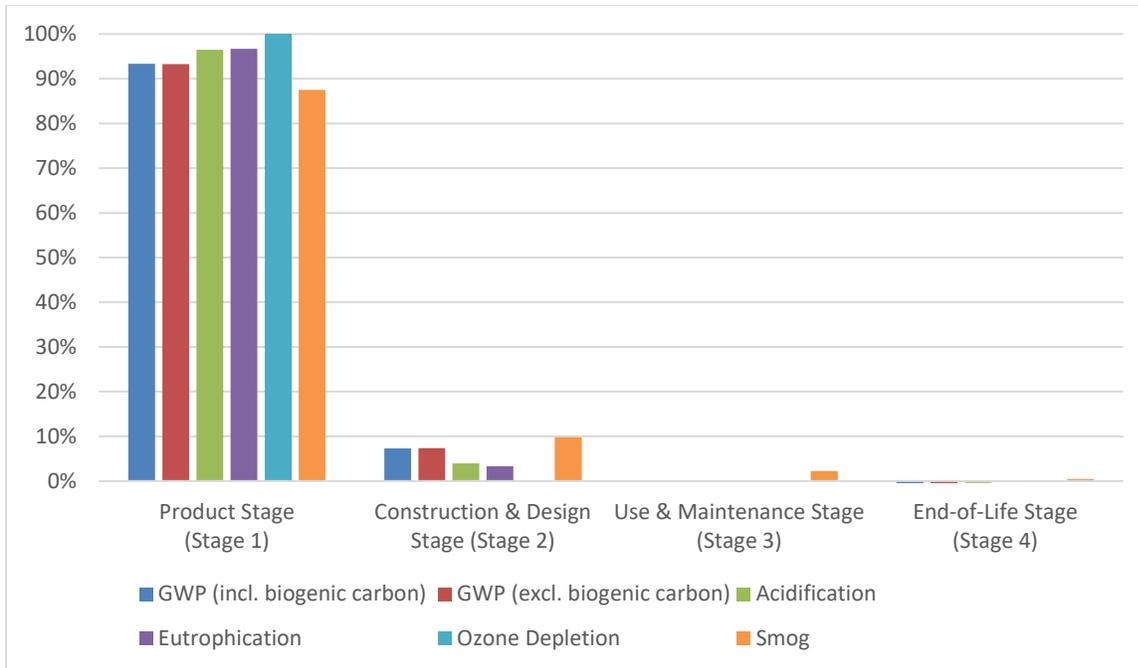
**Figure 2. Impact Category Result Breakdown by ISO 21930 Stage for coating system (as mixed).**
