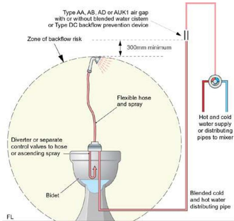
b. be supplied with cold water from an independent distributing pipe serving the bidet only, or a common distributing pipe serving the bidet and which may also serve a WC or urinal flushing cistern at a lower level. See Diagram 4; or
