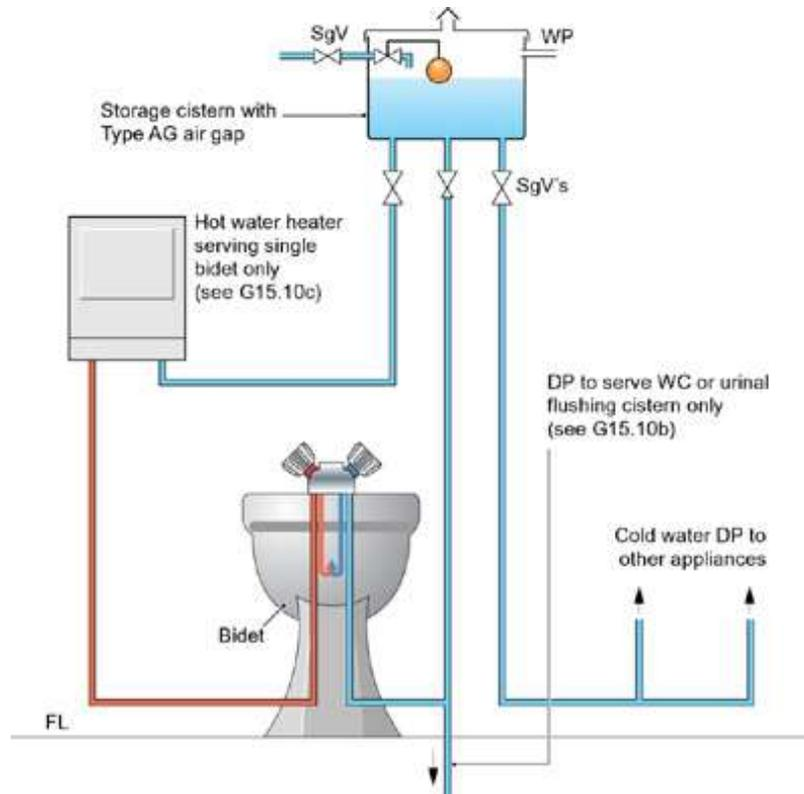
d. where the bidet is at a lower elevation than any other outlets or appliances, be supplied with water from a common cold and/or hot water vented distribution pipe providing that;
